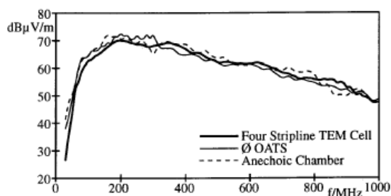
Fig. 13: Four Stripline TEM Cell to 10 m OATS Correlation
