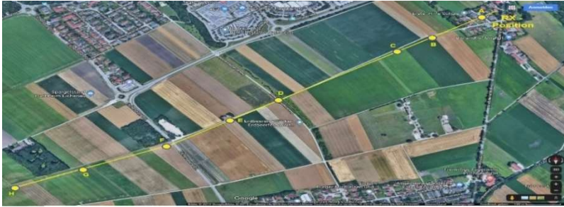
Fig. 5: 8 TX Positions A to H (1.65km H - 46m A) car distances to the RX (up right) 10m high
