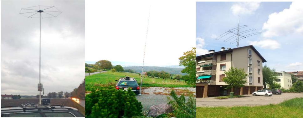
Fig. 3: Two co-polarized 40m verticals, and two non-co-polarized reference test antennas
